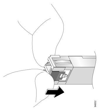
Step 5 With the tab still pushed, carefully pull the SFP module from the port as shown in Figure 28.
